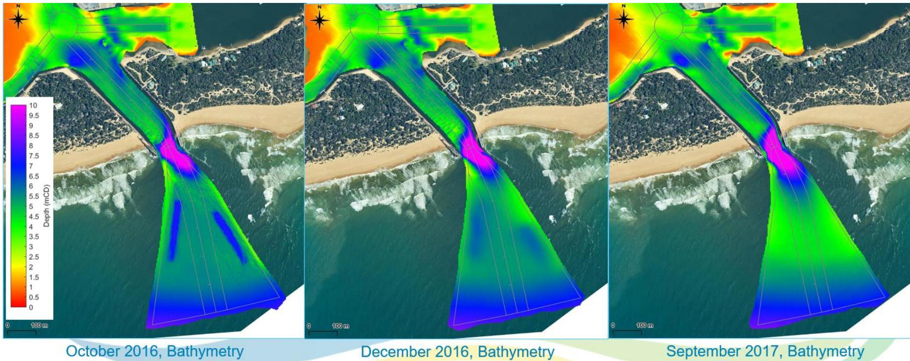
Figure 32: Bathymetry of Bar and Entrance Channel for the 11-month period without dredging following the last dredging works with contracted TSHD Pelican (October 2016) and prior to arrival and operation of Gippsland Ports owned and operated TSHD Tommy Norton in September 2017. (PCS, 2021)
