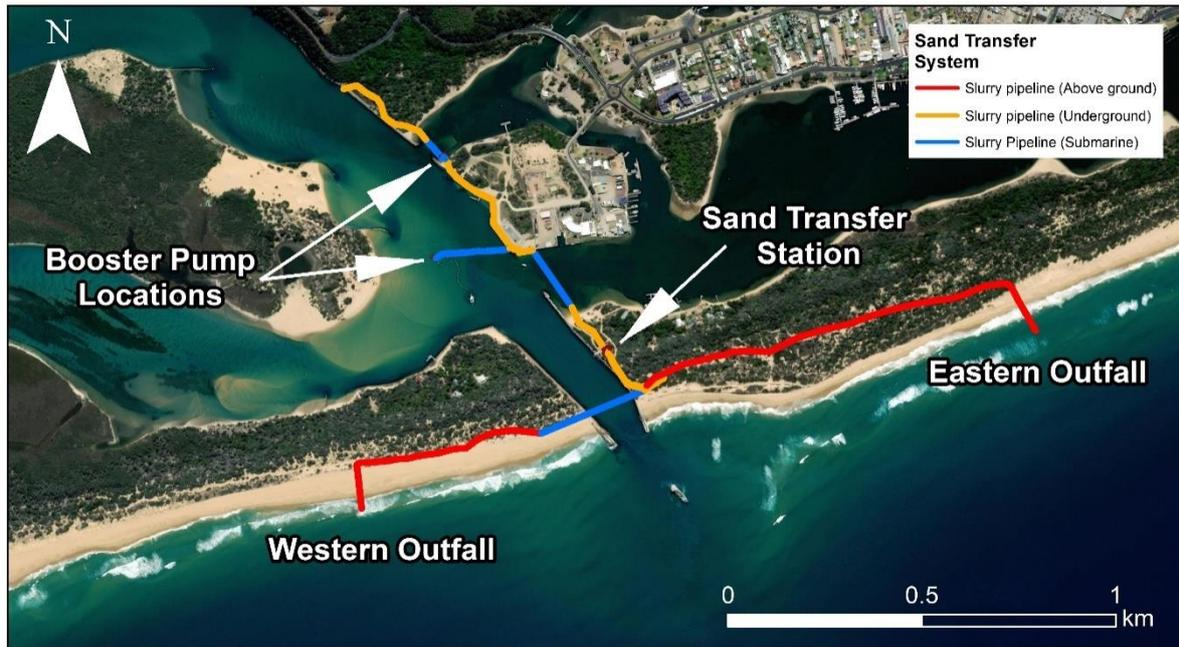
Figure 51: Sand Transfer System infrastructure locations
