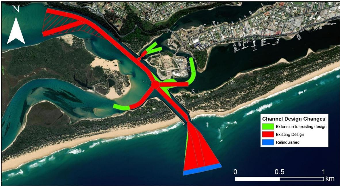
Figure 43: GLOA proposed navigational channel design modifications (2022)
