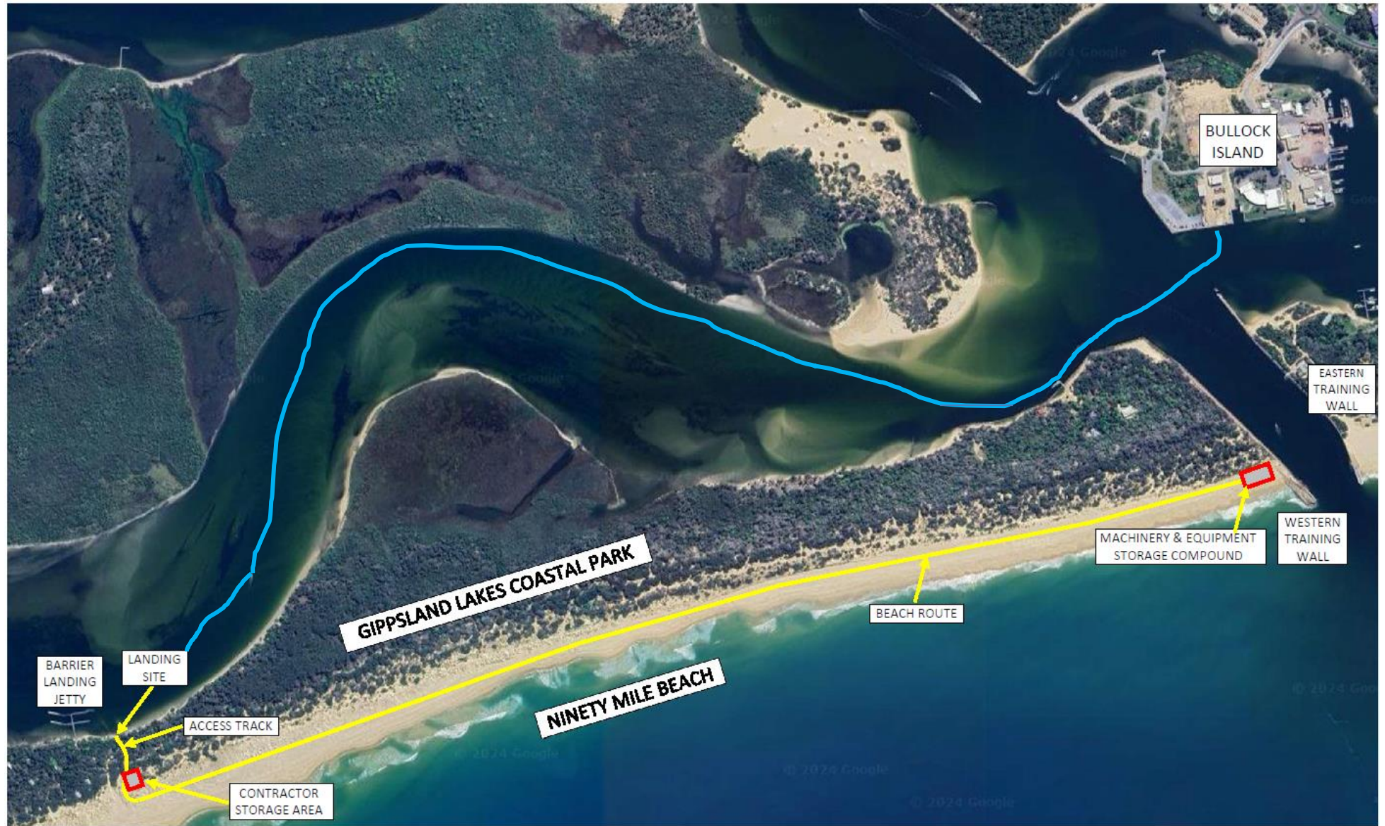
Land based activity areas on Boole Poole Peninsula associated with works on the Western Training Wall
