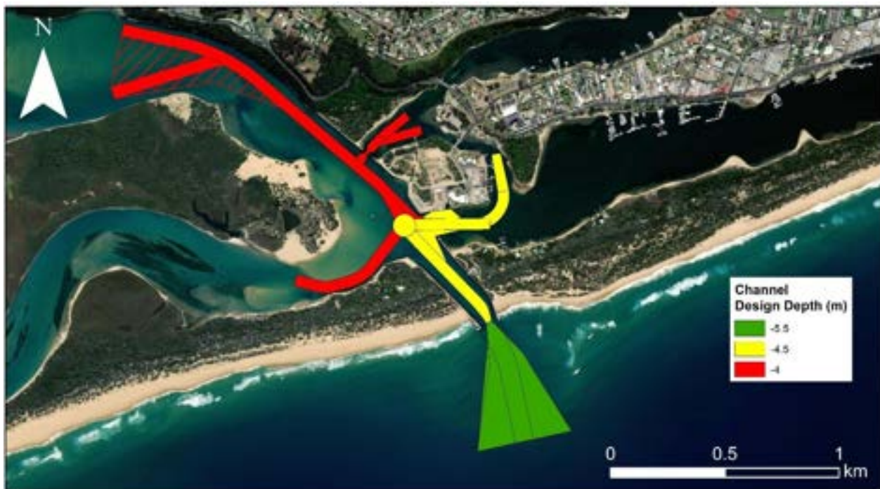
Figure 2. Proposed channel design depths relative to Chart Datum for the future dredged channel configuration.
