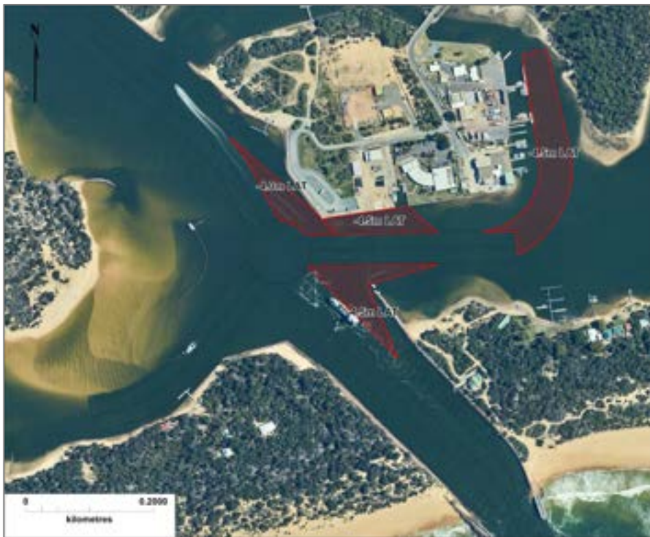
Figure 43. Option IC01 dredge design.
