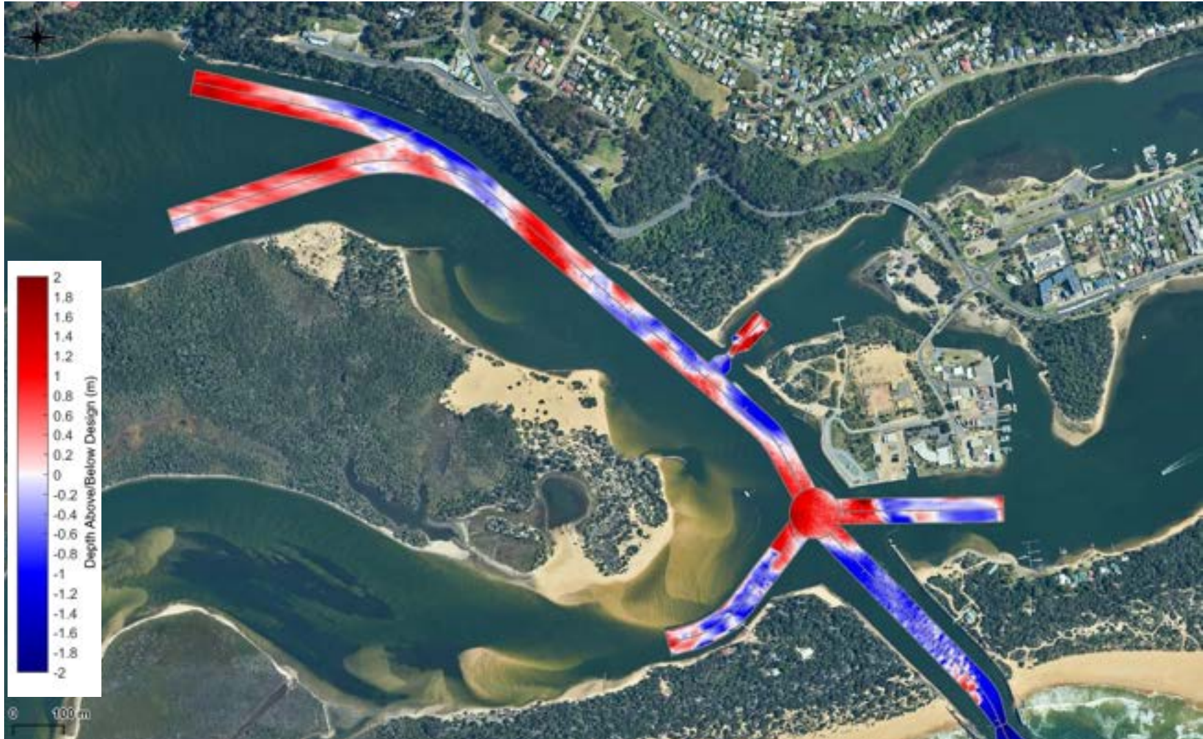
Figure 10. Depth relative to design depths for the Inner Channels in November 2020 (PCS, 2021a). Note: blue is below design depth, red is above design depth.
