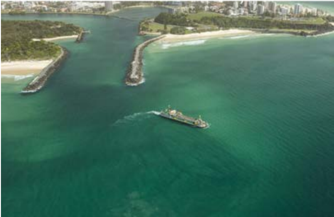
Figure 35. Oblique aerial image showing the TSHD Albatros dredging the Tweed River entrance bar (Dutch Dredging, 2021).
