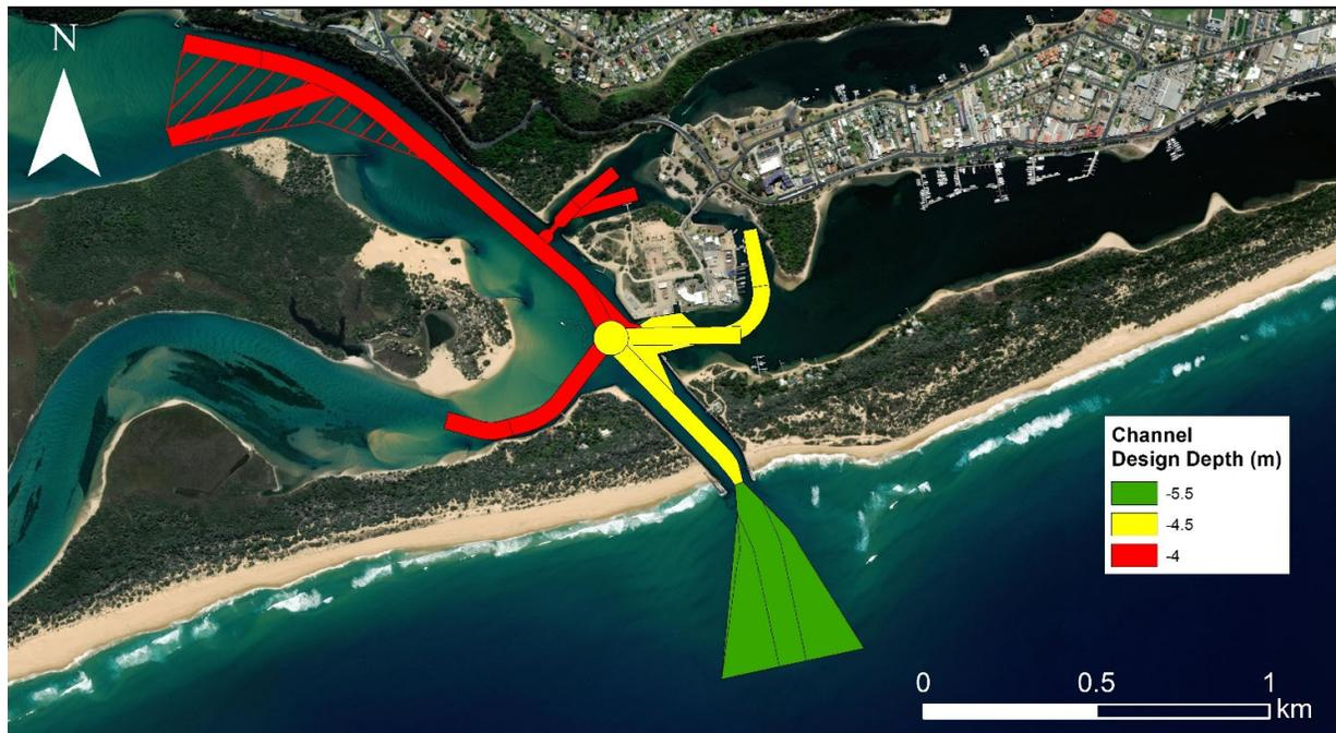
**Figure 4. Channel design depths for the Entrance, Bar, Wedge, Swing Basin and Inner Channels.**
