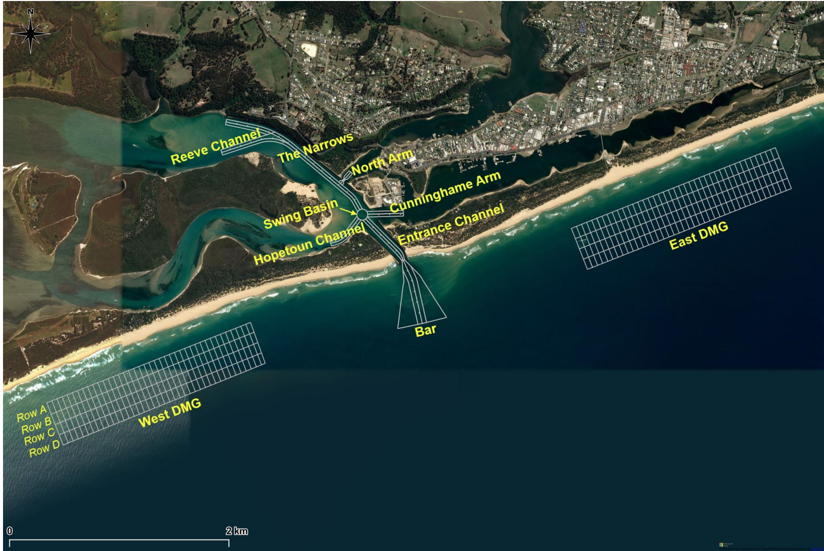
Figure 3. Port of Gippsland Lakes dredged areas and Dredge Material Grounds (DMGs).
