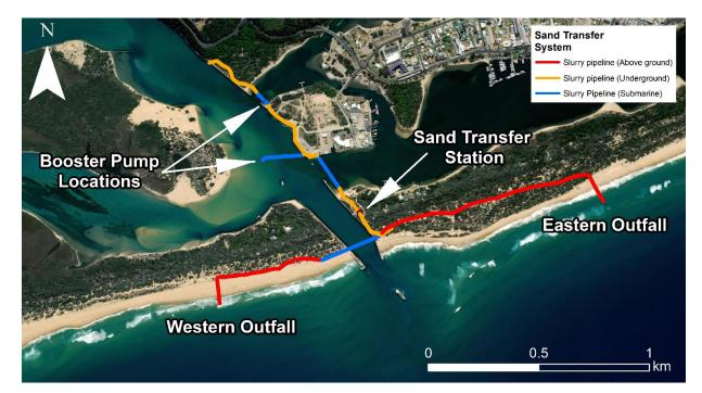
Figure 3. Location of the Sand Transfer System and nearshore outfalls.
