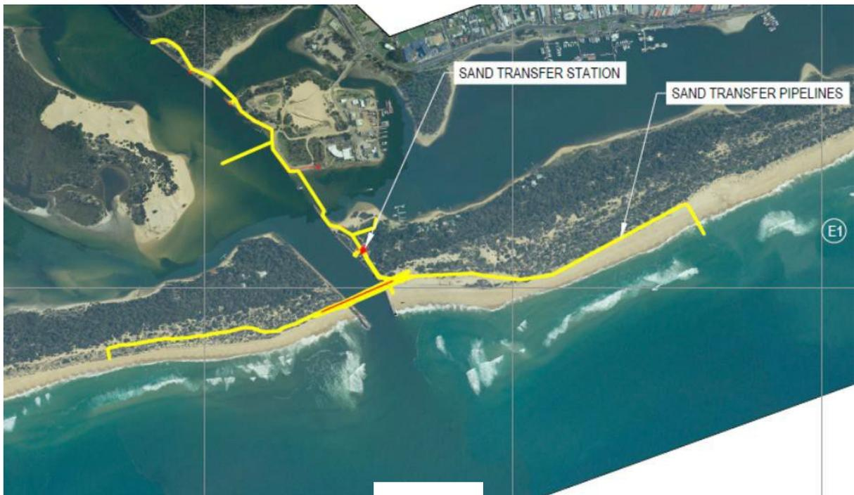
Figure 6: Layout of the Sand Transfer System
