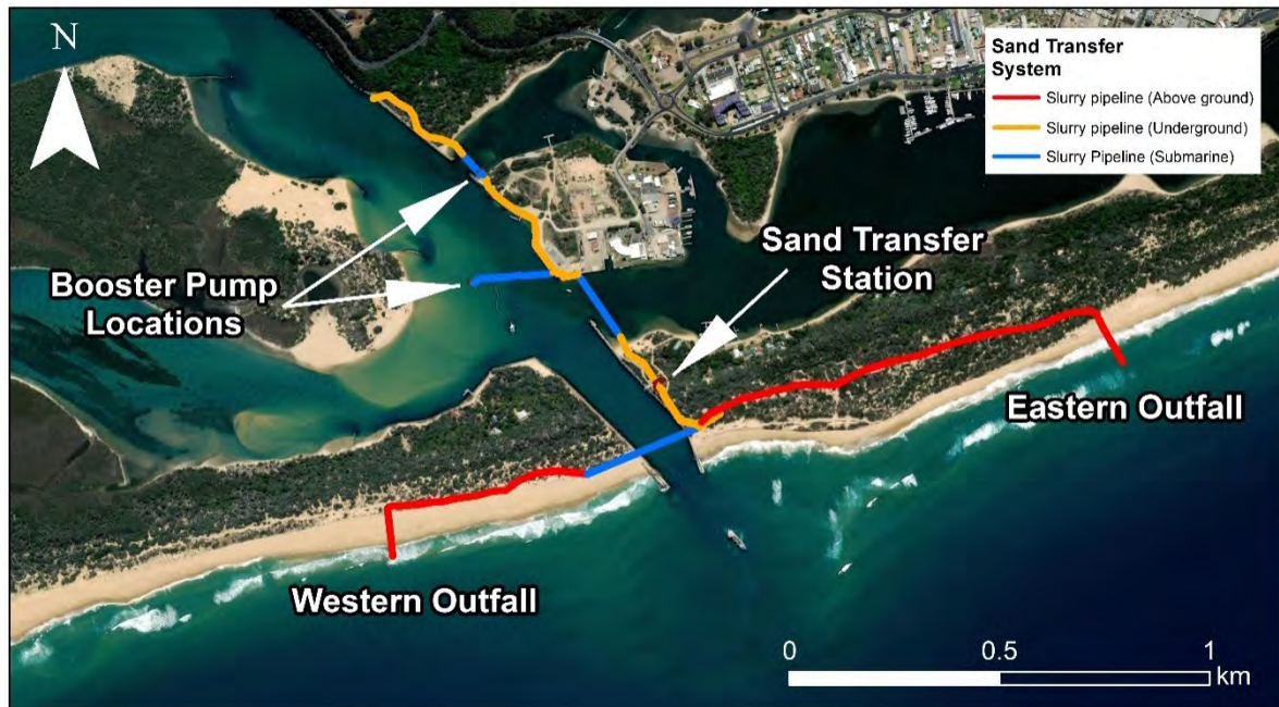
Figure 51: Sand Transfer System infrastructure locations
