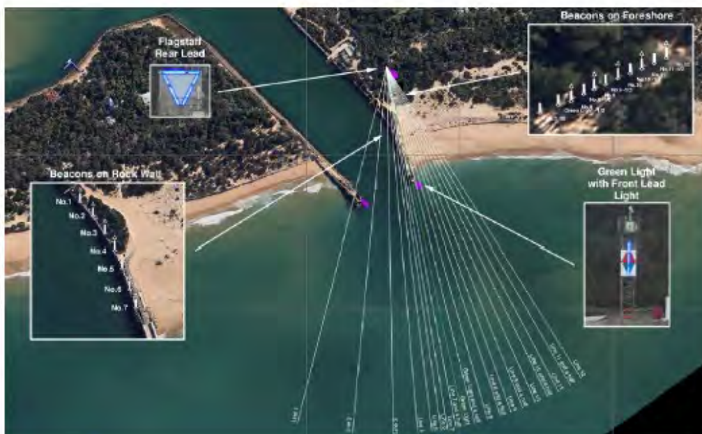
The photo above illustrates the characteristics of the "Flagstaff Rear Lead" triangular blue LED light apex down, and the "Green Light Front Lead" vertical bar LED light. The Green Line indicates the line of approach with the "Leads in Line". The Leading lights are available day and night.
