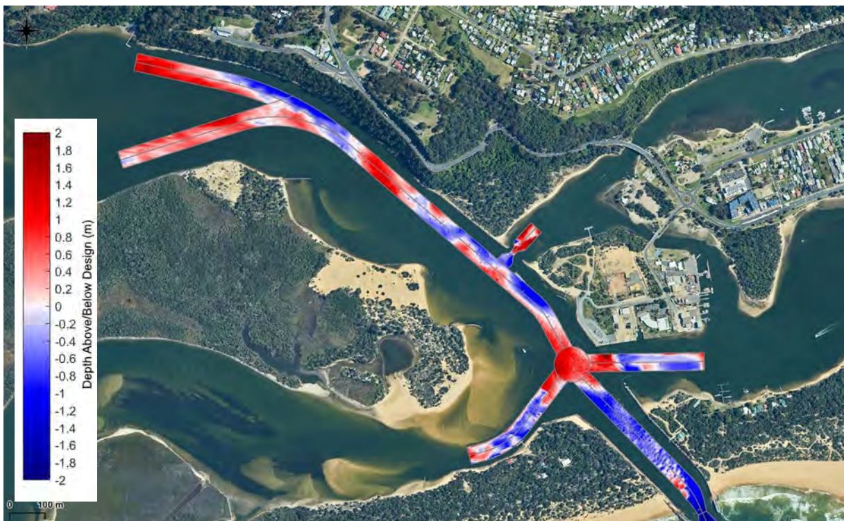
Figure 35: GLOA Inner Channel depths relative to design depths (November 2020) (PCS, 2021)
