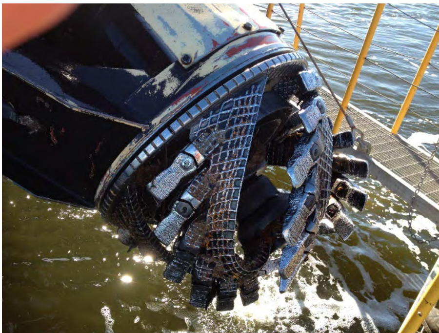
Figure 50: Cutter suction head on Dredger Kalimna
