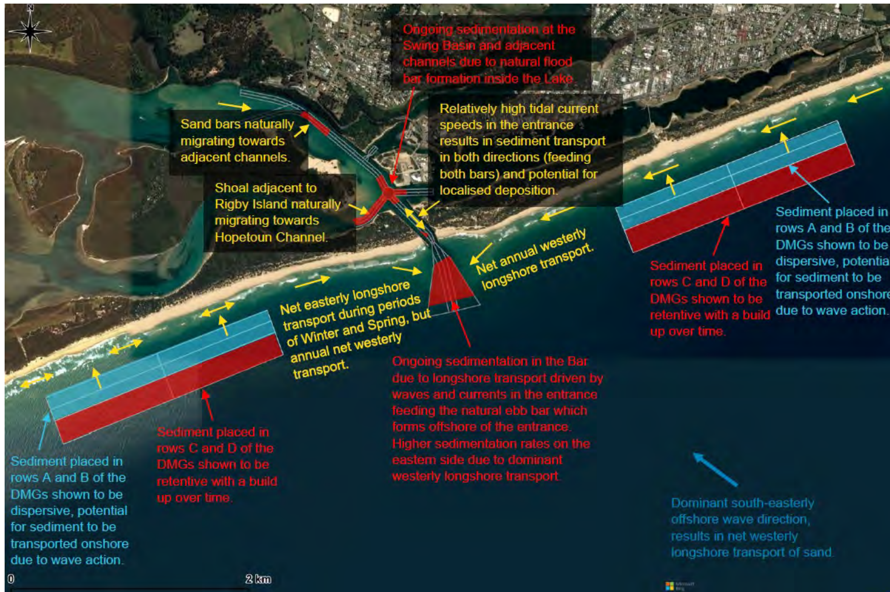
Figure 39: Conceptual sediment transport understanding for Lakes Entrance
